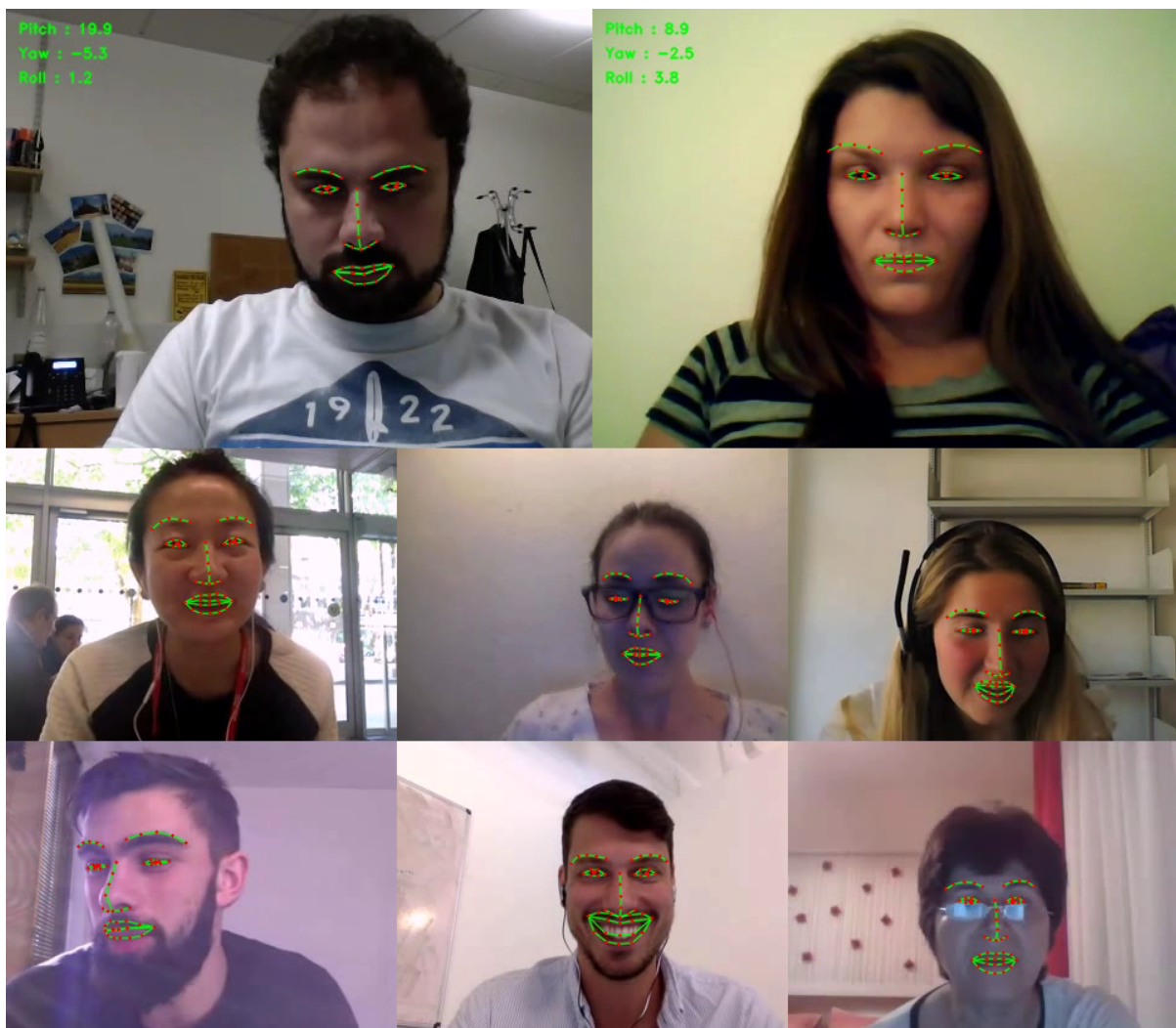
Figure: The automatic facial landmark localisation results obtained using the Chehra tracker (see section 6.2 for details). The top row shows the results on the advert-watching recordings and the two bottom rows show the results on the video-chat recordings.
